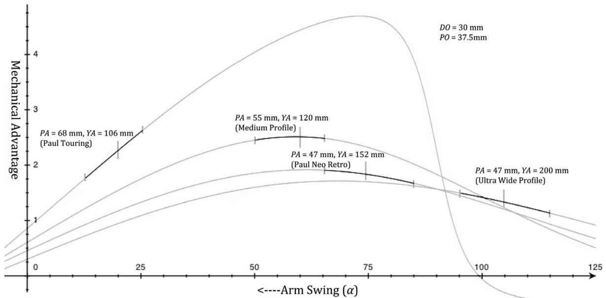
**Figure 3: MA as a Function of Angle ( $\alpha$ ): Straddle Cable Length Fixed**
