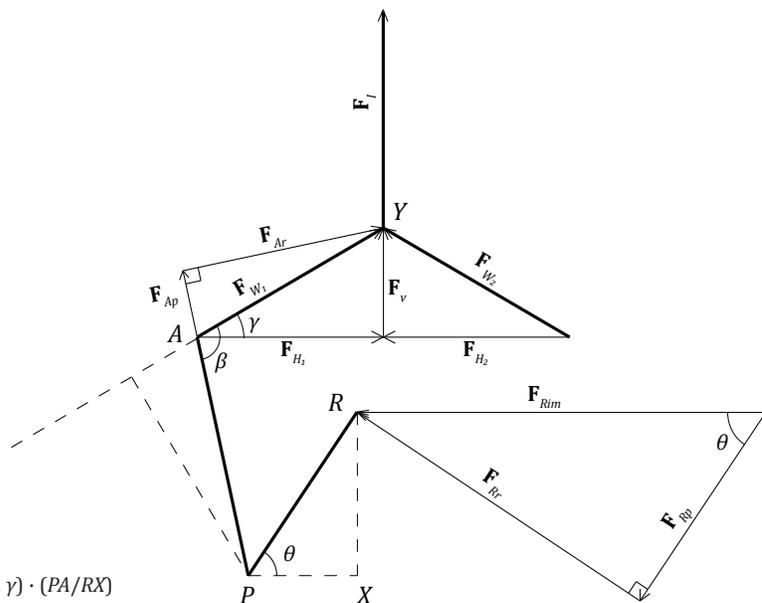
7 Brown states that the MA is inversely proportional to the length PR (not DO). This would be true if PR were striking the rim squarely. Since the pad arm is hitting the rim obliquely, it is the vertical component DO, which is parallel to the face of the rim and perpendicular to the applied force, that is relevant to MA.
